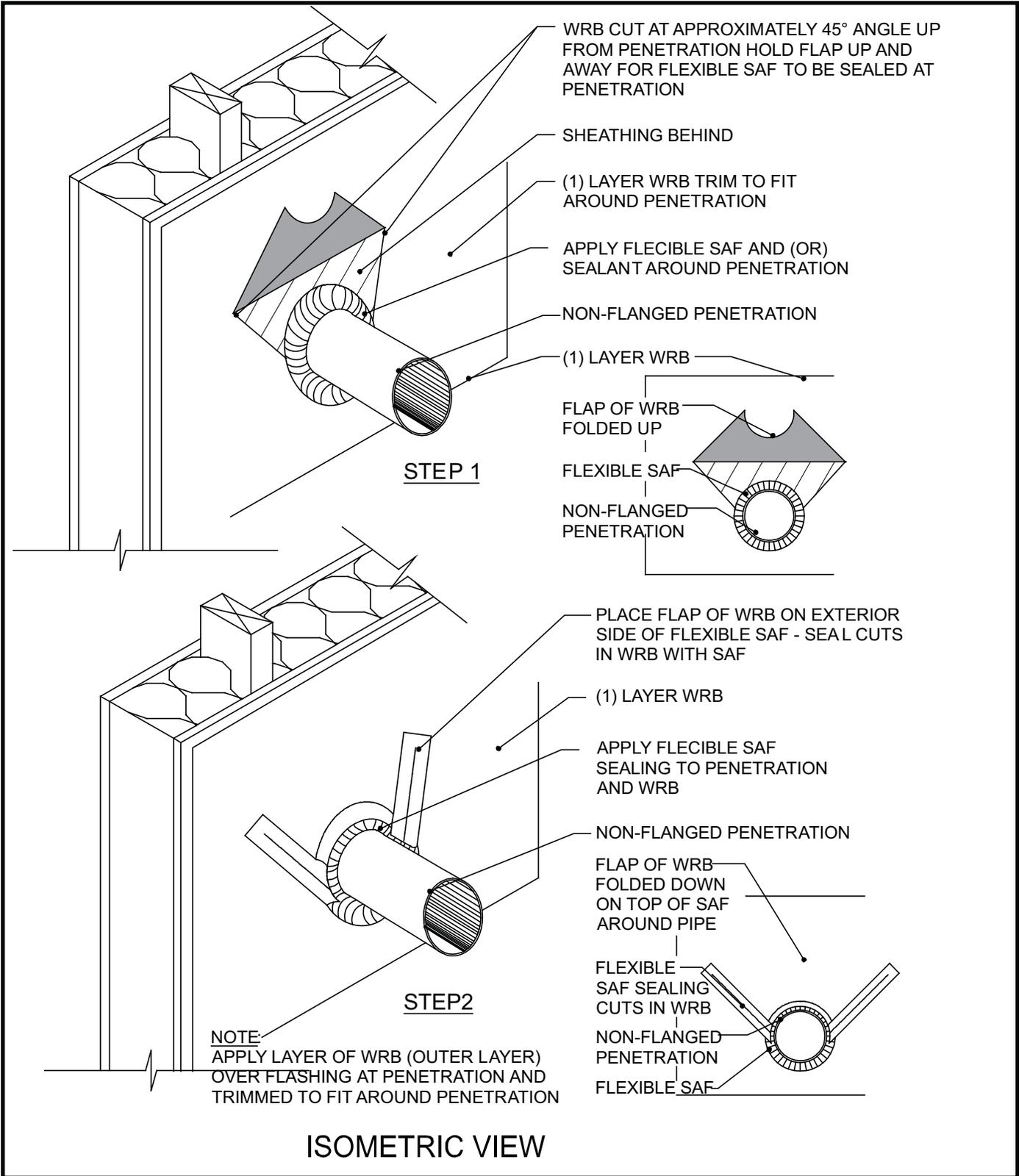
Flexible self-adhered flashing around the penetration and WRB lapped in a watershed fashion help prevent water infiltration.
