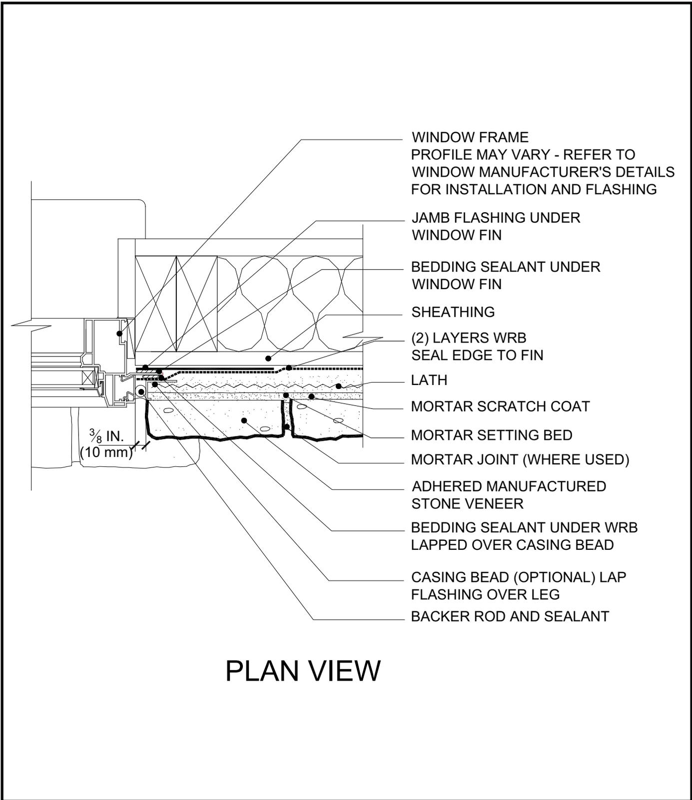
Rough openings must be properly flashed prior to window installation. Backer rod and sealant between the window frame and the adhered manufactured stone veneer allows for movement between the dissimilar materials.
