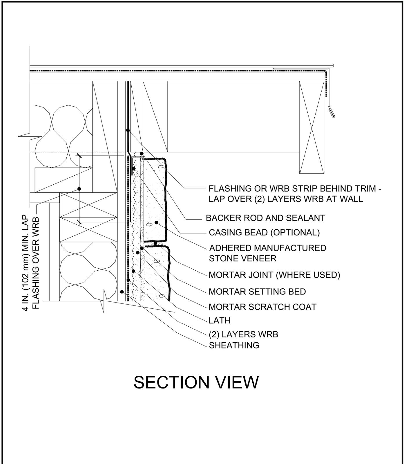
The intent of these details is to limit exposure to wind driven rain.
