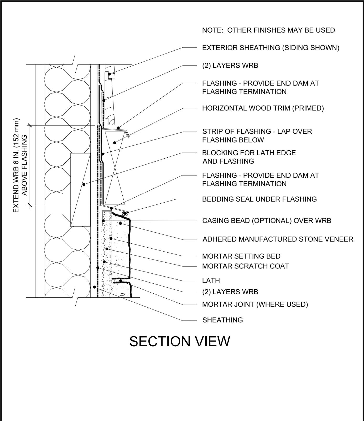
Note: flashing is lapped shingle-fashion with corrosion resistant sheet metal. A bedding seal is used under the corrosion resistant sheet metal next to the adhered manufactured stone veneer.
