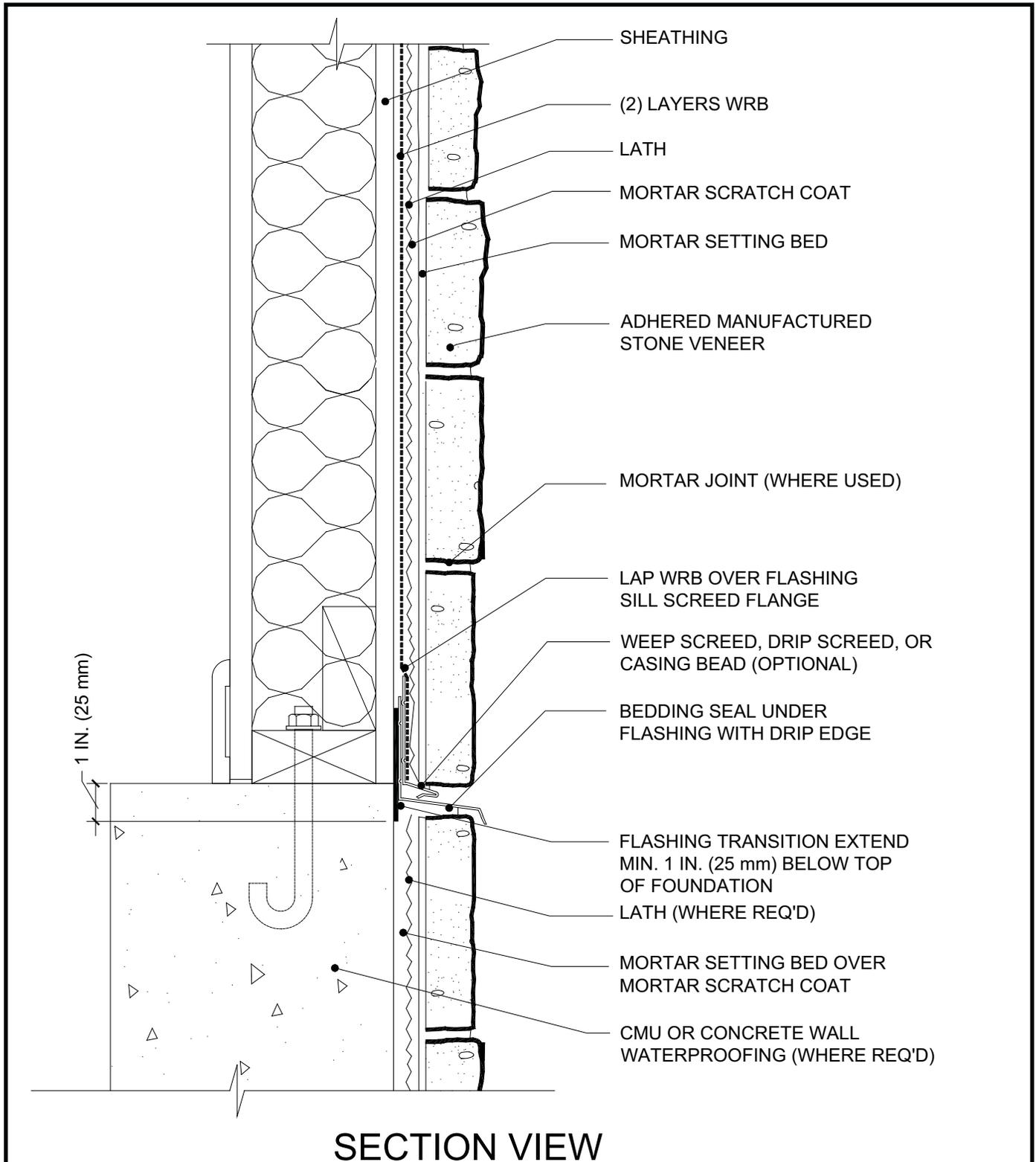
AMSV may continue down the foundation with the incorporation of a flashing transition with careful installation of WRB and flashing.
