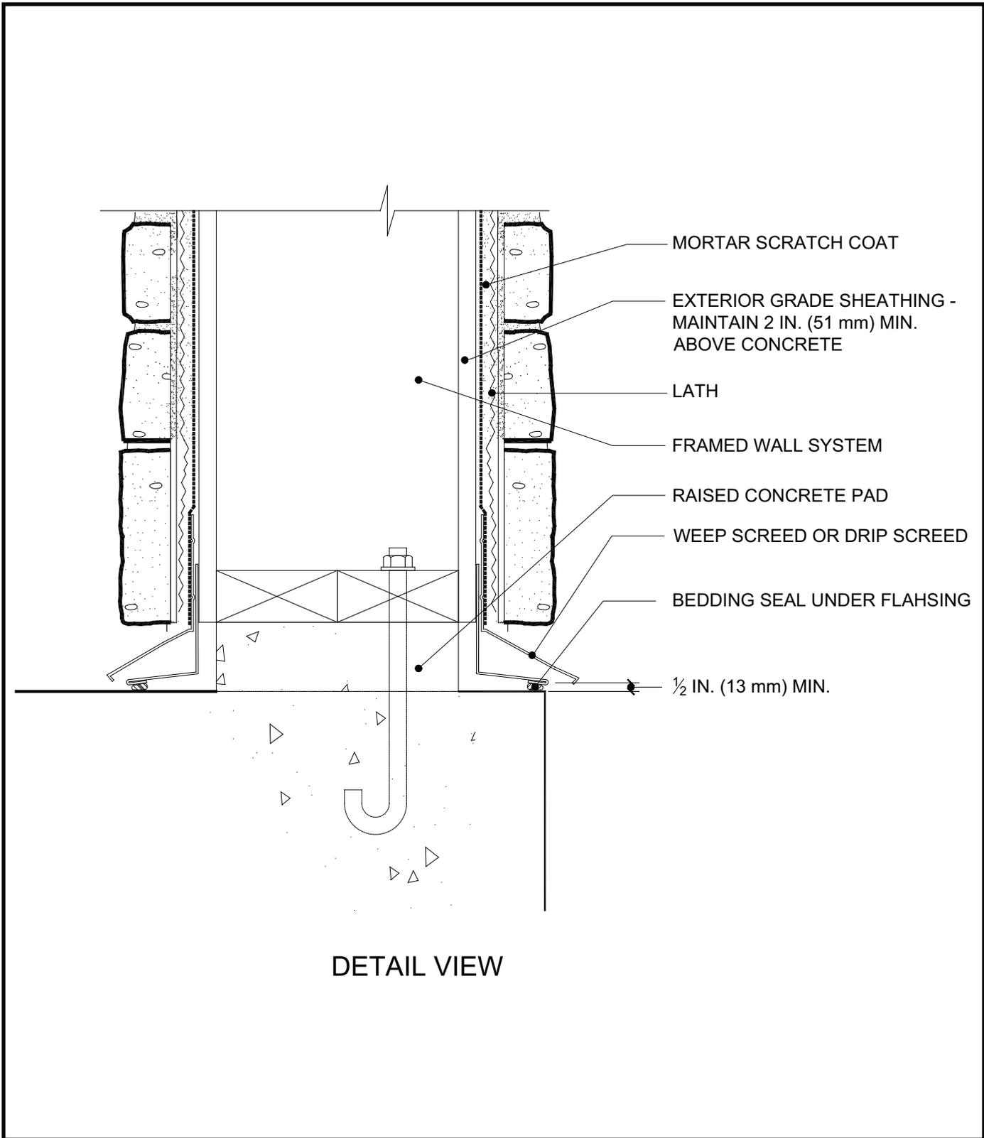
Adhered manufactured stone veneer may overlap the raised concrete pad, but a clearance of one half inch (13 mm) should be maintained at all sides of the base. Do not extend flashing past edge of AMSV.
