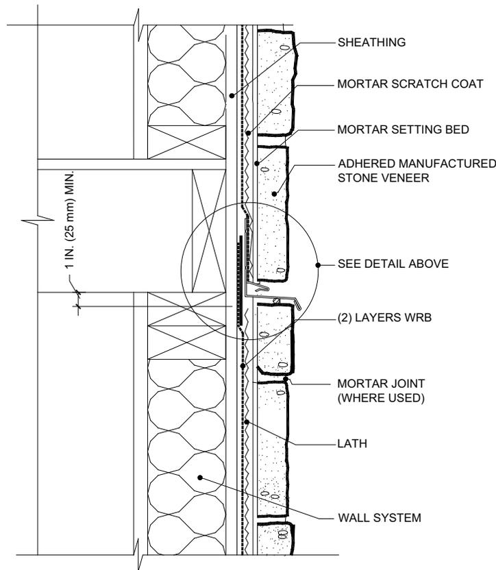
NOTE: FOR GUIDANCE WITH LATH FASTENING SYSTEM REFER TO THE FOAM COALITION WEBSITE, AS WELL AS LATH FASTENER SECTION OF THIS GUIDE. AIR BARRIER, VAPOR BARRIER, WATER-RESISTIVE BARRIER, WATERPROOFING MEMBRANE, FLASHING, LATH ATTACHMENT, Z-CHANNEL, AND INSULATION TYPE AND LOCATIONS TO BE DETERMINED BY DESIGN PROFESSIONAL
