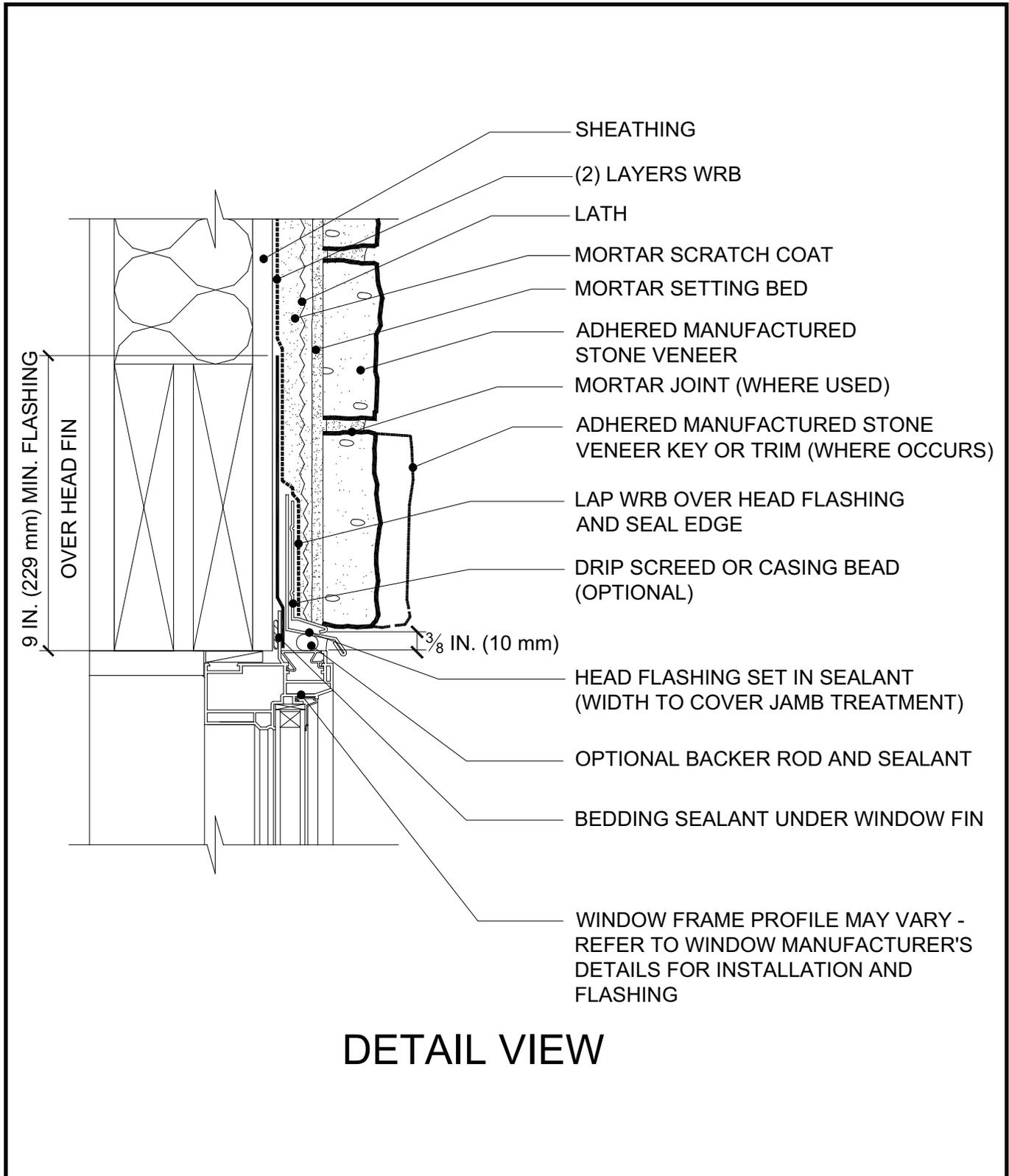
Flashing and WRB installed shingle fashion may be complimented with self-adhered flashing to seal WRB to window frame.
