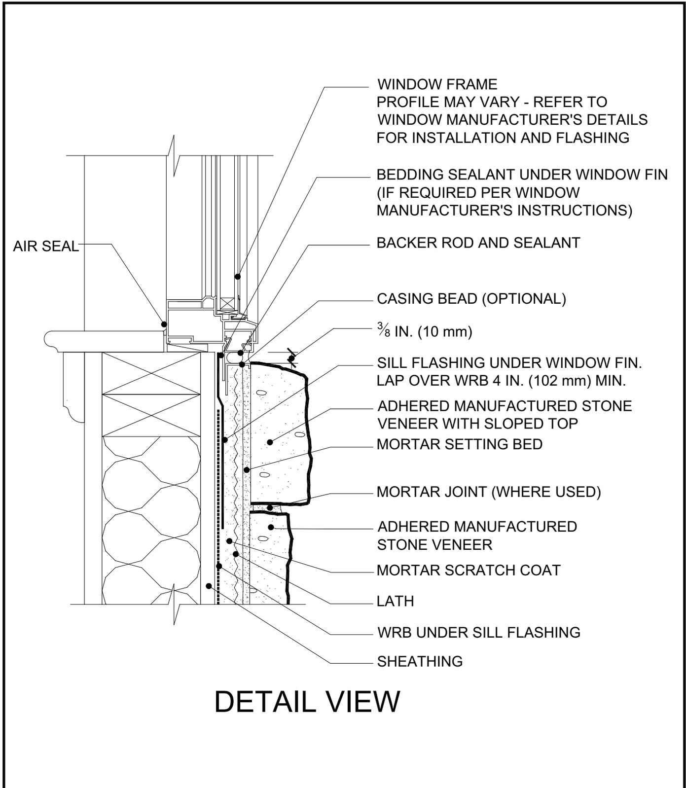
Rough openings must be properly flashed prior to window installation. Tuck water resistive barrier under flashing at sill. Sill flashing should drain to the exterior of the primary WRB or to exterior of adhered manufactured stone veneer.
