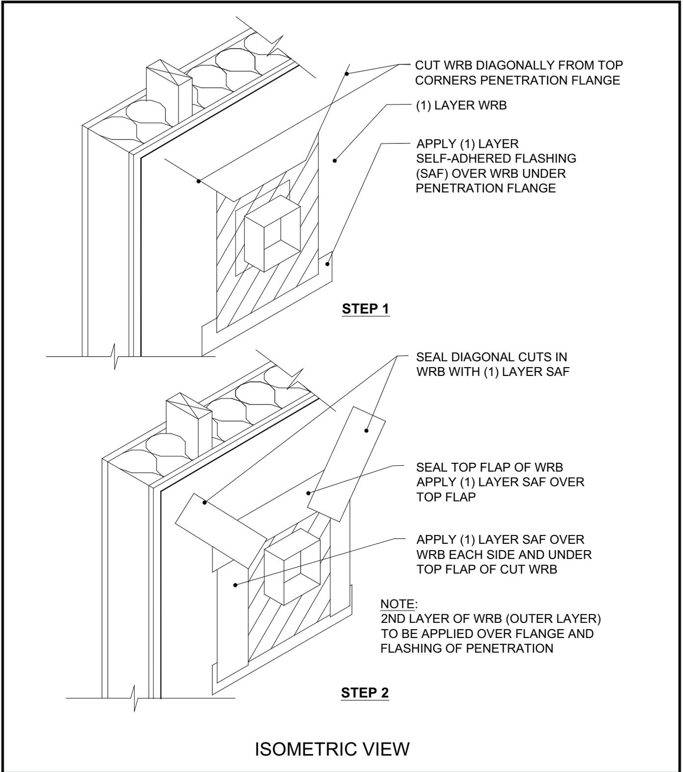
Penetration with flanges can be incorporated into the wall system by applying WRB in a watershed fashion and sealing cuts in the WRB with self-adhered flashing. Drawing illustrates installation with housewrap WRB. Installation with building paper WRB would be similar but instead of 45 degree cuts, fit last piece of WRB on top of flanges and tuck under WRB course above penetration (similar to Step 2 in Fig. 31.).
