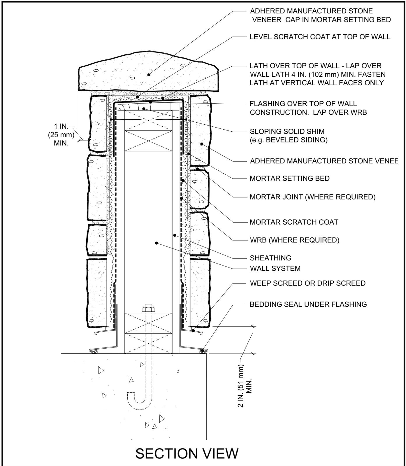
A sloping solid shim should top the wall under the flashing and lath. Flashing should lap the top of the wall. Lath should lap over the top of the wall but be fastened only to vertical wall faces.
