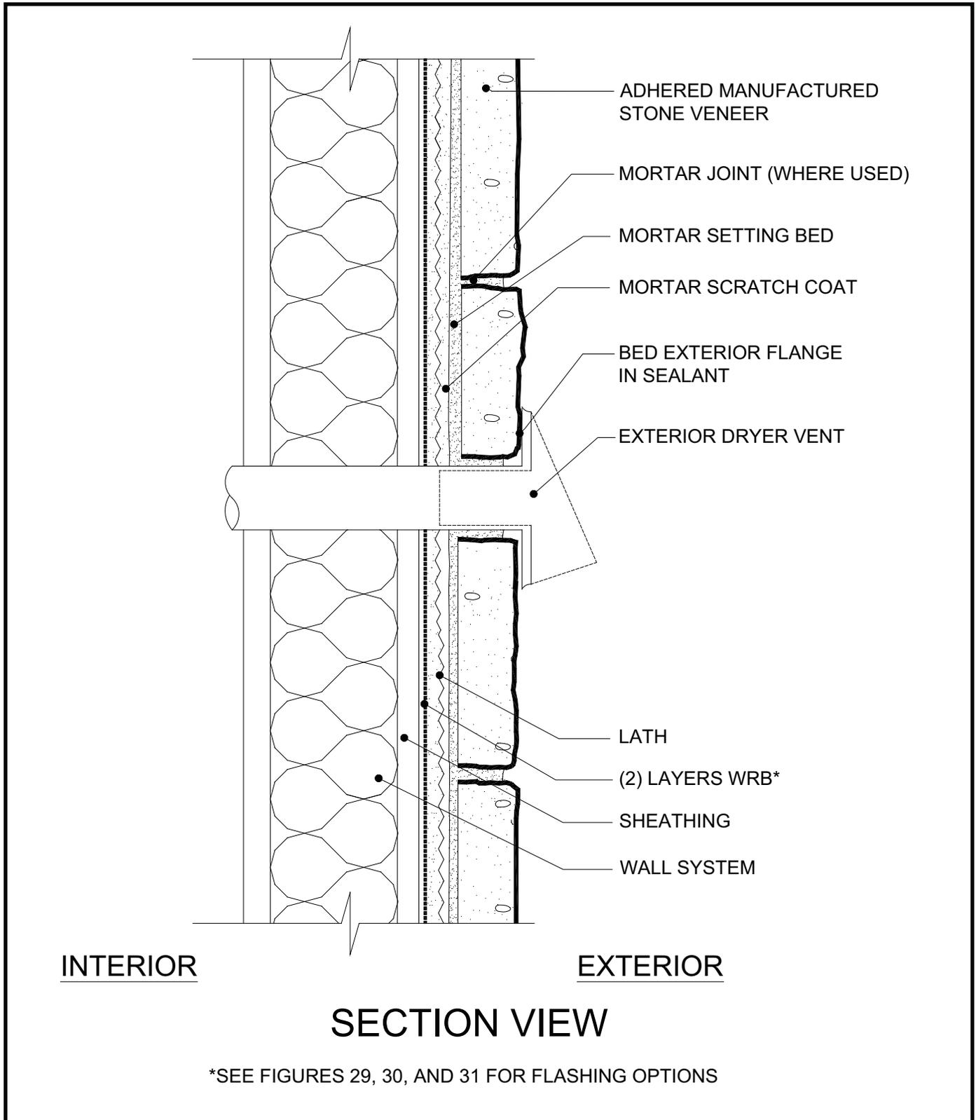
Bed all covers, flanges, and escutcheons in sealant before fastening to the wall.
